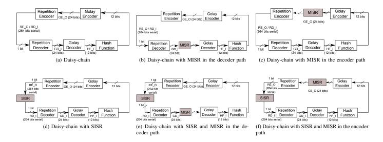
Fig. 4: Daisy-chain for a FE - different constructions
