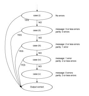
Fig. 2: Golay Decoder state-machine
