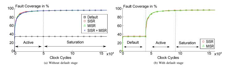
Fig. 5: Fault coverage of Fuzzy Extractor Daisy-chain test method versus clock cycles
