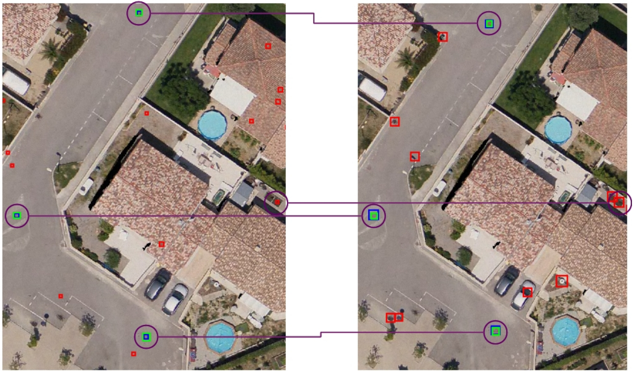
Fig. 5. The two figures represent the results obtained with the circular filter on the left and the machine learning method on the right. The red rectangles are the true negatives, the blue rectangles are the true positives and the green rectangles are the ground truth. The lines connect the two common results between two approaches. The testing image is at 4 cm resolution.
