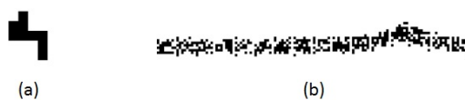
Figure 2. (a) Multiple Cell Upset as a result of a particle induced current that spreads over several neighbouring cells. (b) Multiple Cell Upset as a result of a micro-SEL.
