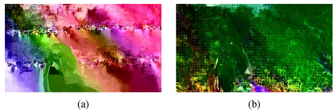
Fig. 9. Known plaintext attack for kimono #0: (a) Encrypted frame: PSNR (YUV) = {10.12, 20.65, 14.23} dB, (b) Video frame with encrypted bits set to 0: PSNR (YUV) = {11.12, 20.19, 14.69} dB.
