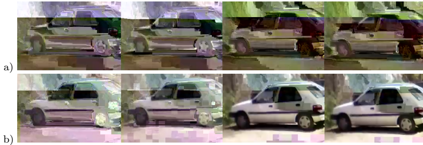
Fig. 11 A ROI of the ar-drone video sequence: a) A reduced selective encryption of only the I frame of a 2-frame GoP, b) A reduced selective a encryption of only the I frame of a 4-frame GoP.
