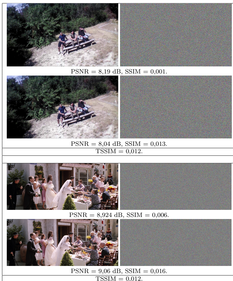
Fig. 7 Full encryption of two successive frames of ar-drone (on top right) and movie (on bottom right) with the corresponding original frames (on left). The PSNR and the SSIM between the encrypted frame and the original one is indicated below each case. Moreover, TSSIM between the successive frames is indicated below the second frames for each video sequence.
