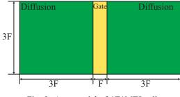
Fig. 2: Area model of 1T1MTJ cell
