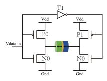
Fig. 4: PMA STT-MRAM write circuitry
