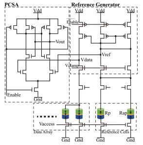
Fig. 3: Reference generator and sense amplifier circuitry [17] [18]
