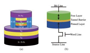
Fig. 1: (a) Perpendicular anisotropy magnetic tunneling junction structure (b) The commonly used 1T1MTJ cell structure
