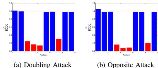
Fig. 10: Results obtained by combining the proposed detection technique (BCDC and k-means) and LNR filtering
