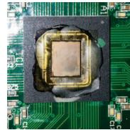
Fig. 7. Decapsulated FPGA and injector used during experimental campaigns
