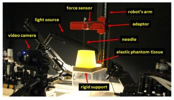
Fig. 3. The Raven II platform. Original architecture was customized in order to perform needle insertion experiment.
