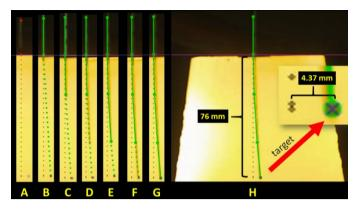
Fig. 5. Sequential insertion of semi-rigid needle into soft PVC Phantom tissue. The target is defined online (A), followed of offline needle deflection prediction (B). A loop of insertions and needle tip updates are performed (C-F) until the needle tip reaches the target depth (G-H).
