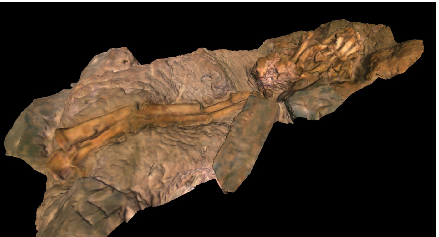
Figure 6. The corresponding 3D reconstruction (535,668 vertices / 1,067,723 triangles) of the left arm based on 18 views (each around 100 to 400,000 points) acquired by the NextEngine scanner.
