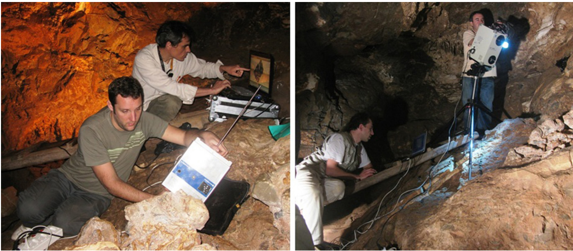
Figure 3. The 3D digitizers in situ: left the NextEngine HD; right: the Minolta VIVID 910.
