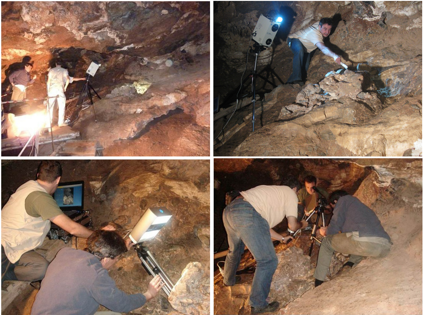
Figure 4. Some practical difficulties: dealing with uncontrolled lighting, measuring and tuning the adequate depth of field, and positioning the scanner tripod on a chaotic surface without touching the fossil.
