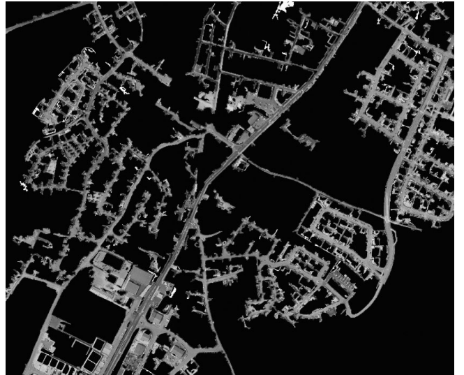
Fig. 3. Roads detection using grey-level threshold and extraction of the biggest connected components.
