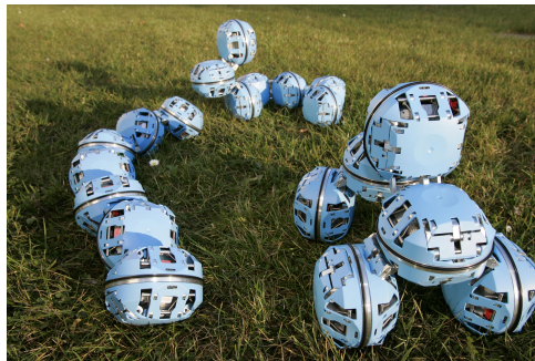
Figure 27: ATRON [55], an example of modular, self-reconfigurable robot
