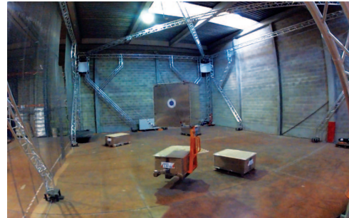
Fig. 2. LIRMM/TECNALIA CoGiRO suspended CDPR prototype.
