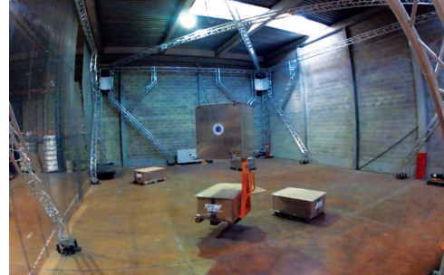
Fig. 2. LIRMM/TECNALIA CoGiRO suspended CDPR prototype.
