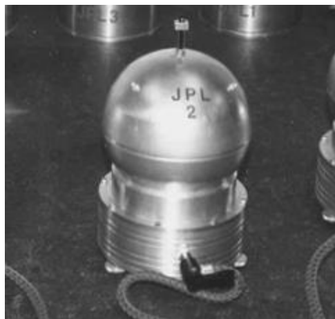
Figure 10. Experimental hollow air bearing platform in University of California, Los Angeles/California Institute of Technology model spacecraft spheres [11]
