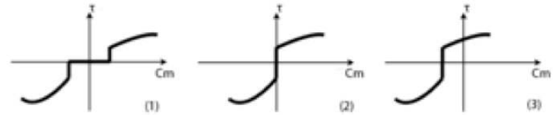
Figure 6. Management of dead zones (1: nominal ; 2 : contraction ; 3 : setting operating point)
