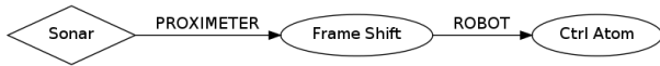
Fig. 3. With the Atom Datatype, we are forced to express explicitly the shift from PROXIMETER to ROBOT frame.
