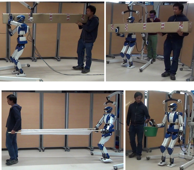
Figure 11. Experiments with the HRP-4 carrying various objects in collaboration with a human.
