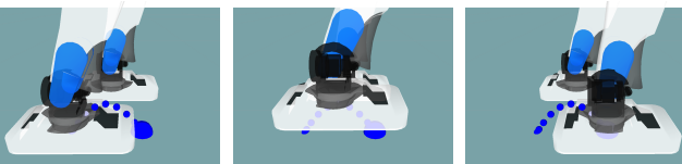
Figure 5. Parameterized swing foot trajectory.
