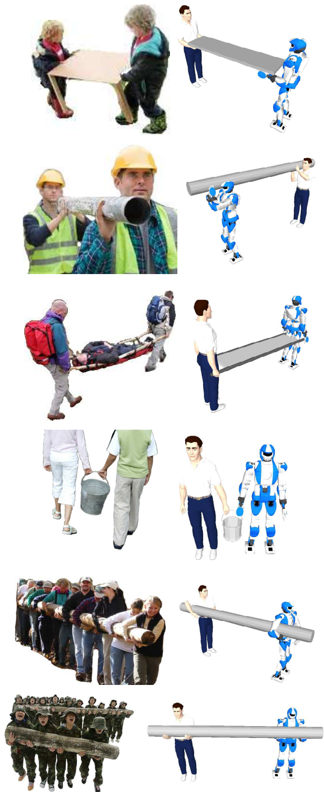
Fig. 1. Collaborative carrying examples (left), with a human avatar and a humanoid robot mimicking the corresponding postures (right).
