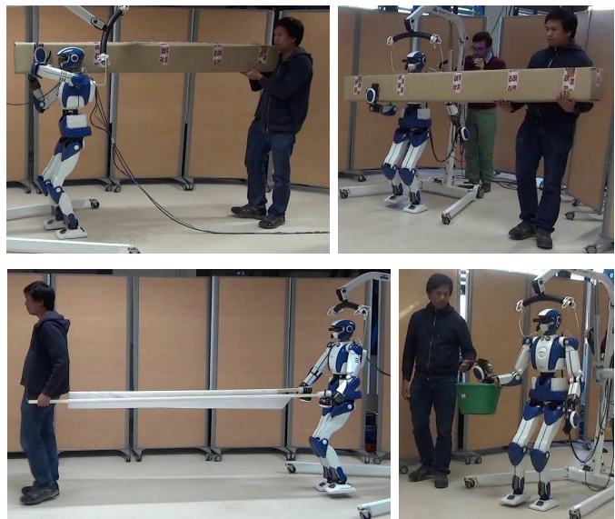
Fig. 10. Experiments with HRP-4 carrying various objects with a human. Top: 15N carton box, bottom left: 13N stretcher, bottom right: 8N bucket
