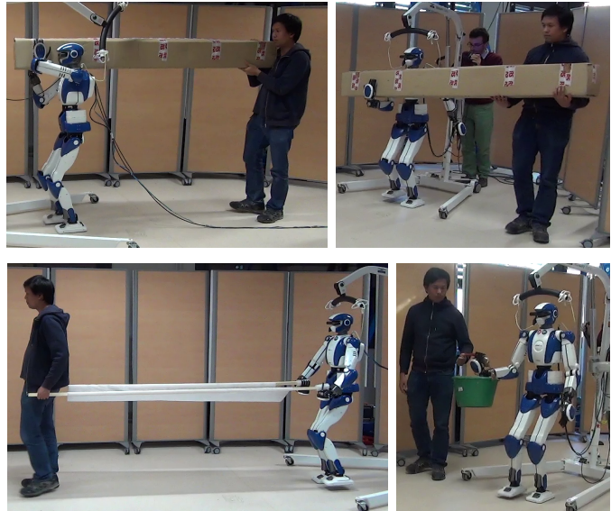
Fig. 9. Experiments with HRP-4 carrying various objects with a human. Top left: 15\text{N} carton box. Top right: 15\text{N} carton box (for this experiment please refer to time 0:23 of the attached video; the robot starts in a half-sitting posture with its right arm preparing to hold the box; while the robot grasps the box, the left arm motion, which was not programmed ad hoc, results from the weight of the box and from the CoM/ZMP equilibrium tasks). Bottom left: 13\text{N} stretcher. Bottom right: 8\text{N} bucket.
