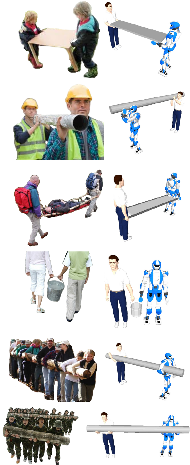
Fig. 1. Collaborative carrying examples (left), with a human avatar and a humanoid robot mimicking the corresponding postures (right). These figures are merely illustrative, since some postures may be unfeasible due to joint range limitations in the real HRP-4 humanoid platform (e.g., the fifth posture from the top is unfeasible on humanoid robot HRP-4, because of the body grasp configuration).
