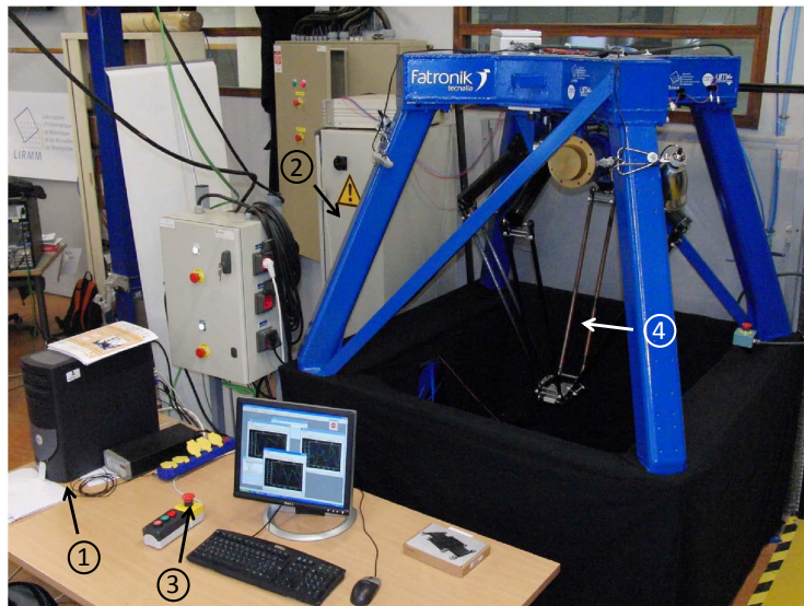
Figure 10: Par2 parallel manipulator experimental setup
