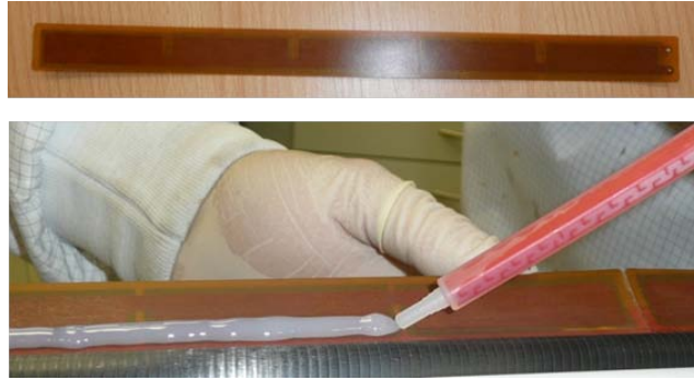
Figure 27: Piezo patch (top) and its fixation process (bottom)
