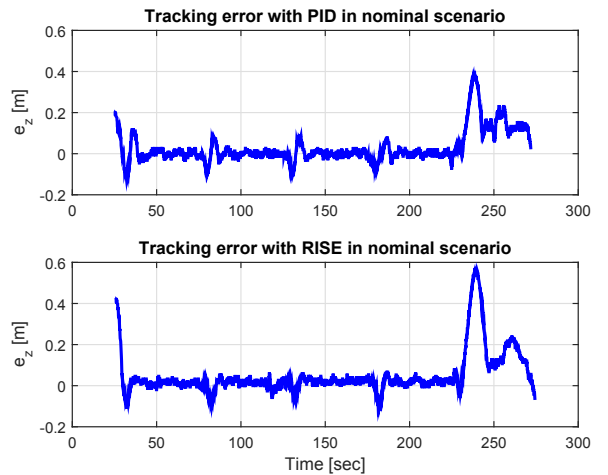
Fig. 5. Evolution of depth tracking errors versus time for nominal case. Top: For the PID controller, bottom: For RISE controller.
