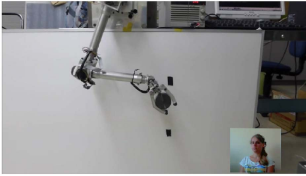
Fig. 9. Subject performing the online control of multi-DOF robot in a simultaneous way by using co-adaptive BMI. The black dots indicate the targets for the subjects in the vertical plane.
