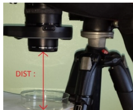
Fig. 1. Image acquisition setup for the CiradRiceSeed dataset
