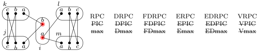
Fig. 6 A CFN that satisfies all RPC consistencies but does not satisfy any PIC consistency. i < j < k < l < m . Every value of i satisfies RPC consistencies because it has more than 2 full (hence simple) arc supports in c_{ik}, c_{ij}, c_{il}, c_{im} . The problem does not satisfy any PIC consistency because of variable i (value (i, a) is not simply (hence not fully) extensible to triangle \Delta_{ilm} while (i, b) is not simply (hence not fully) extensible to triangle \Delta_{ijk} ).
