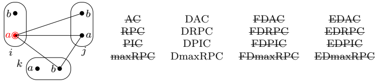
Fig. 9 A CFN which is directional consistent ( i > j > k ) but is non-directional inconsistent. The problem is not AC because (i, a) has no arc support in c_{ij} . However, the problem is DAC because every value of j and k has full arc support in c_{ji}, c_{ki} . Moreover, the problem is DmaxRPC (hence DPIC, DRPC) because every value of j and k can be fully extended on the triangle (in the triangle \Delta_{ijk} , only the smallest variable k and c_{ki}, c_{kj} are concerned by triangle-based directional consistencies).
