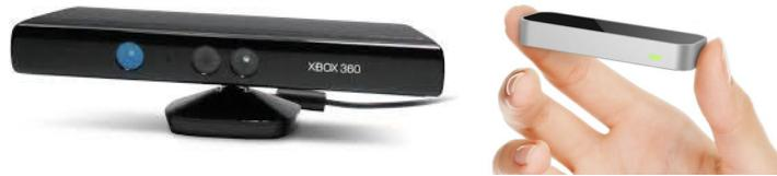
**Fig. 4.** Gesture recognition devices: left Microsoft Kinect, right Leap Motion
