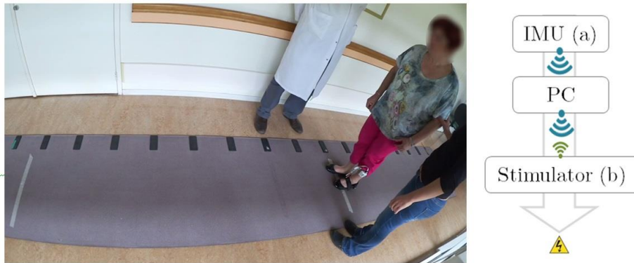
Fig 3. The subject is equipped with an inertial measurement unit (a) and a wirelessly programmable stimulator (b) connected through a PC.
