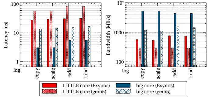
Fig. 5: Latency and bandwidth of the main memory controller.
