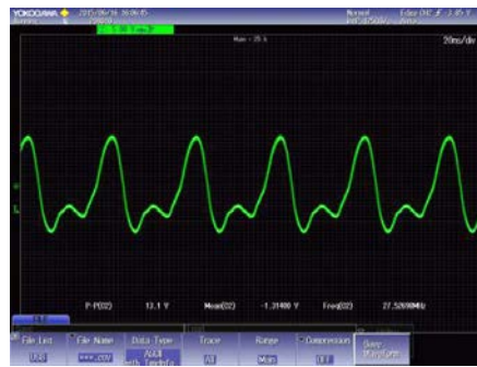
Fig. 7. Measured \Delta V' voltage oscillations from the conditioner prototype.
