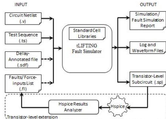
Figure 1. tLIFTING architecture
