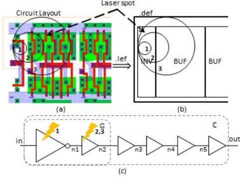
**Figure 4.** Abstract the illuminated sub-circuit from circuit layout to logic-level netlist. (a) Transistors illuminated by 3 different size laser spots; (b) Corresponding gates; (c) Sub-circuit with the perturbed gates
