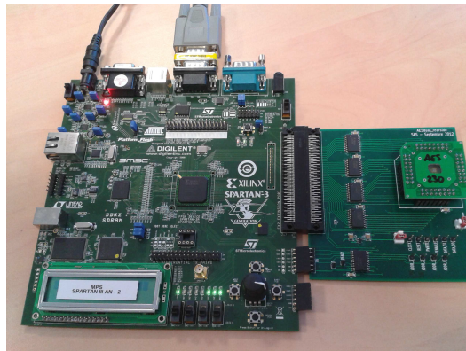
Fig. 10. FPGA board linked with the PCB board and the AES for backside injection
