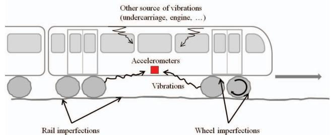
Fig. 2: Sources of vibrations measured by the accelerometers
