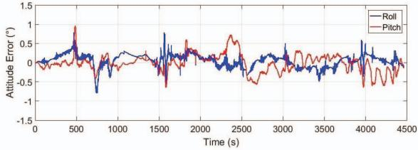
Fig. 5: Train attitude errors during the experimentation
