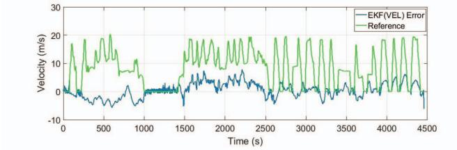
Fig. 6: Train velocity error observed during the experimentation
