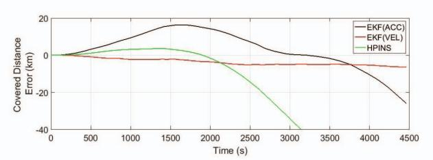
Fig. 7: Train covered distance error observed during the experimentation
