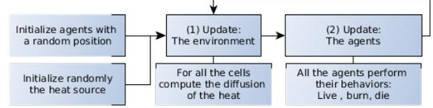
Figure 4: Fire simulation
