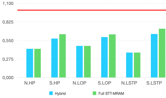
Fig. 12. 1 MB 16-way cache read latency (relative to classic SRAM)
