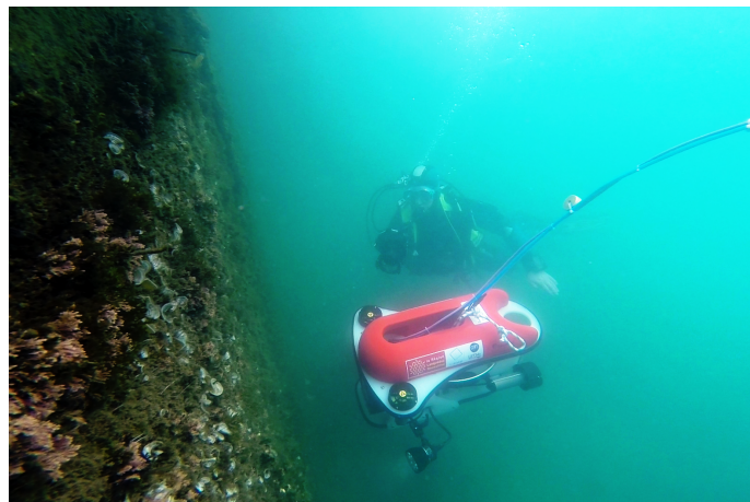
Figure 1: View of the L2ROV underwater vehicle. Its six thrusters allow precise control of its 6 degrees of freedom
