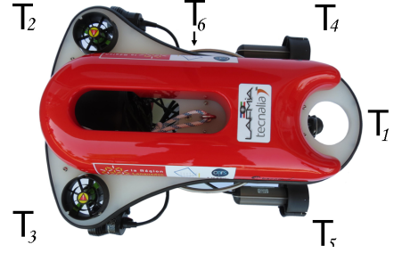
Figure 2: L2ROV: View of forces generated by the thrusters to perform the translational and rotational motions.
