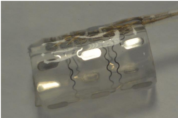
Fig 1. 12-poles multipolar cuff electrode
