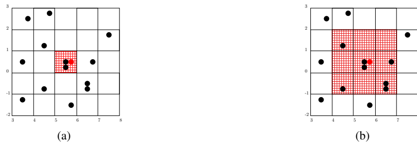
Fig. 3: Query processing in RadiusSketch. Each mapper identifies the cell that correspond to a query and emits the IDs of the corresponding time series (a). If there is not enough information the mapper does a broader search in the adjacent cells (b).
