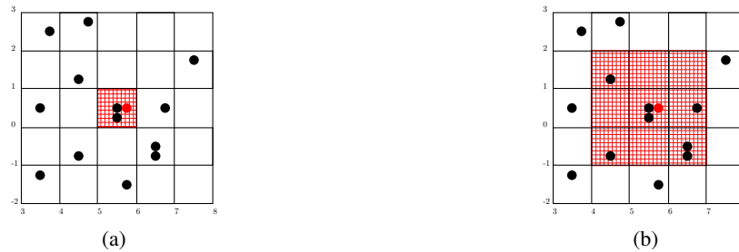
Fig. 3: Query processing in RadiusSketch. Each mapper identifies the cell that correspond to a query and emits the IDs of the corresponding time series (a). If there is not enough information the mapper does a broader search in the adjacent cells (b).
