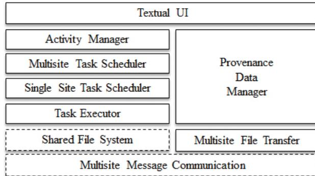
Fig. 5: **Multisite Layered Architecture.**
