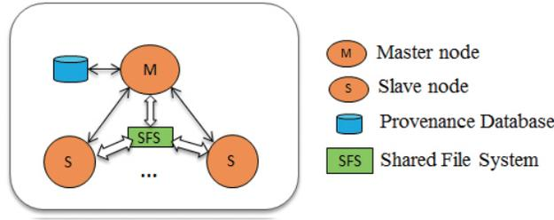
Fig. 1: **Architecture of single site Chiron.**
