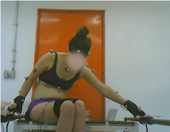
Figure 1: Experimental set-up. The gloves embed pressure sensors. It is possible to see the markers over the subject body, which are captured by the motion capture system. The benches are next to each other, with a 10^\circ angle between them. The legs are constrained to keep them for falling to the sides.
