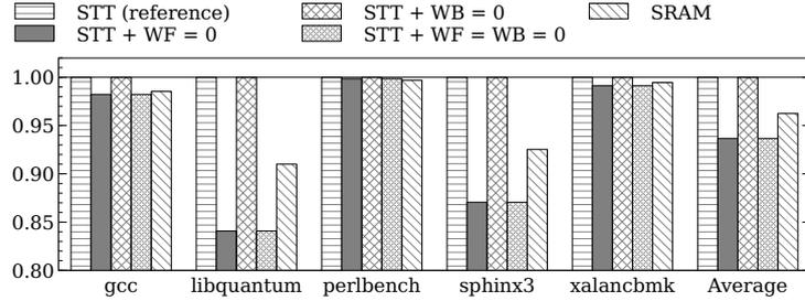
(a) *Write-back* (WB) and *write-fill* (WF) effects on performances normalized to baseline STT-MRAM
