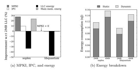
Fig. 1: Evaluation of 2MB and 4MB LLC for soplex and libquantum
