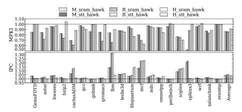
Fig. 6: Performance impact of Hawkeye normalized to LRU
