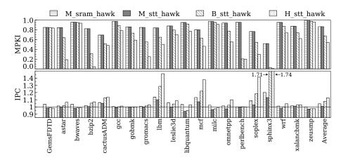
Fig. 5: MPKI (top) and IPC (bottom) with Hawkeye normalized to M\_sram\_lru
