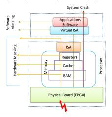
Fig. 1. System Layers and Fault Propagation
