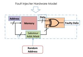
Fig. 3. Fault Injector Hardware Model
