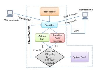
Fig. 5. Work flow diagram of the FPGA-based Fault Injector
