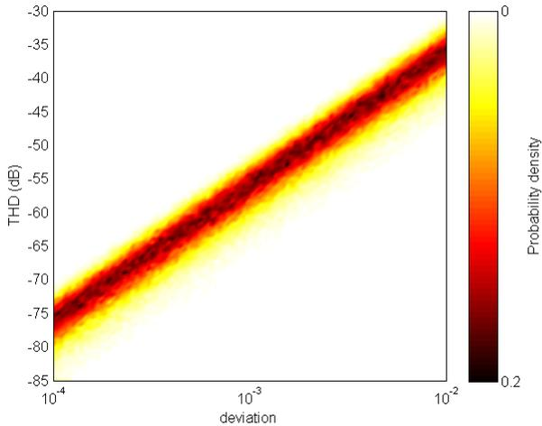
Fig. 7. Harmonic distortion ratio variations due to varying phase-shift error Monte-Carlo results for a sine-wave signal generated using square-wave signals with various phase shifts for six signals  $M = 6$
