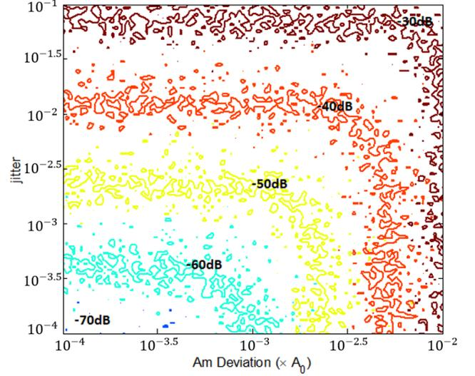
Fig. 14. Harmonic distortion ratio of a sine-wave generated using square-wave signals with various amplitudes deviations and affected by various level of jitter
