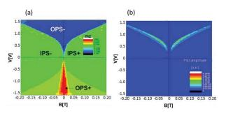
Fig. 3. (a) Static voltage-field diagram of states of free-layer magnetization calculated by taking into account the second order easy-axis magnetic anisotropy. The colour code shows the out of plane mz component of the free layer magnetization. The simulations have been performed for a temperature of 100K; (b) Dynamic voltage-field diagram of states of the free-layer magnetization. The colour code shows the power spectral density amplitude variation.
