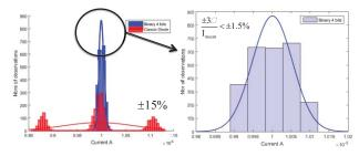
Fig. 7. Impact of process variations on a basic current source (red bars on the left graph) and after calibration using a 4-bits tunable current source (blue bars on the left graph). Closed view of current variations after calibration (blue bars on the right graph).
