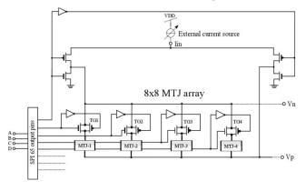
Fig. 6. Schematic view of the designed 8x8 MTJ switch array
