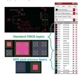
Fig. 5. Layout facilities in the PDK: on the top left, the schematic of the MSS allowing to describe the circuit for electrical simulation. In the middle left, automatic via generation. In the bottom left, the layout of the MSS device and in the right, the Layer Selection Window in Cadence showing the additional layers for the magnetic post-process.
