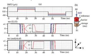
Fig. 4. Comparision of the compact model strategies: the first graph represents the pusle of writing current, whose amplitude is varied. The second one corresponds to the model based on LLG equations, where we can see the expected precessions of the switching and the last one shows the results of the model based on Neel-Brown's and Suns' theories. The models are tuned to give the same results in terms of switching durations
